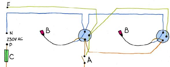
Three Plate Ceiling Rose - wiring the lights – as shown
