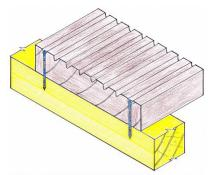
Show how to fix wooden decking to the joists to ensure that the decking does not warp or bow, especially during wet weather – Typical details
