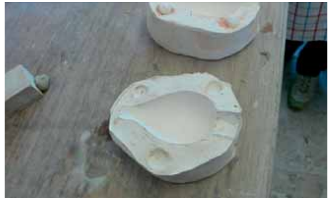
8. Lightly rub the surface with soap and place the object in the mould. Seal the edges with vaseline. Build up another wall of clay to frame the mould and pour the plaster as before.
