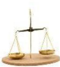
A beam balance is any balance where the beam is horizontal when equal weights are in both pans/sides.
