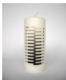
A candle clock is a candle marked with regular time intervals. Candles burn at a constant rate so as the candle melts, you can calculate how much time has elapsed. The thicker the candle, the longer it will burn, so to measure shorter time periods, use a thinner candle. To calibrate a candle, take two identical candles and a stop watch. Line up the candles exactly.
