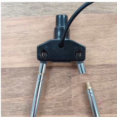
2. Use supplied bracket to set antenna legs to 120 degrees. Orientate North to South when in final position.
