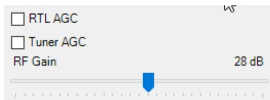
The AGCs used in the RTL-SDR are designed to be used with wideband DVB-T signals, and do not work very well with narrowband signals. We recommend using manual gain control at all times to optimize the gain of a signal, however for casual browsing turning on Tuner AGC may suffice. RTL AGC is almost never used as it tends to just introduce a lot of unwanted noise.
