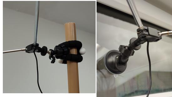
**Set both your antenna legs to a length of 53.4cm, 120° apart, parallel to the ground (Horizontal). The “point” of the V should point North.**
